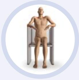
**Too Low** - A seat that is too low will not support the thighs and will increase pressure to the ischial tuberosities and coccyx.
